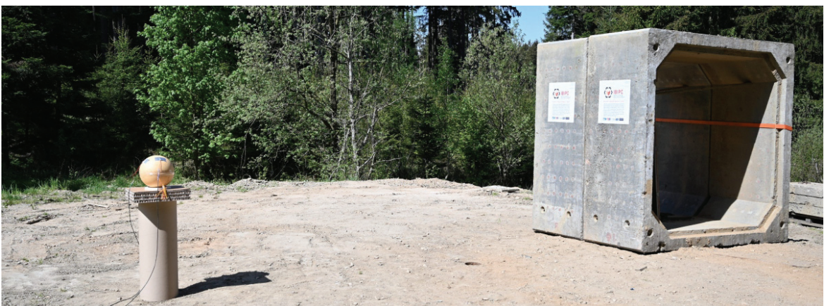
Preparation of test plates and Bunker element for blast and shrapnel resistance tests.
