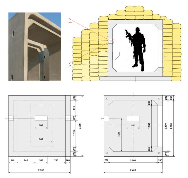
To increase the effectiveness of the protection, it is beneficial to partially embed it in the ground as part of the trench system and to reinforce the protection by lining it with natural material. Variably fitted universal building segment with embrasures, observations slits, entrance hole. Advantage of quick assembly and modular assembly to create a complex defence system.
