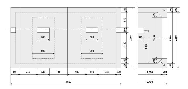
To increase the effectiveness of the protection, it is beneficial to partially embed it in the ground as part of the trench system and to reinforce the protection by lining it with natural material. Variably fitted universal building segment with embrasures, observations slits, entrance hole. Advantage of quick assembly and modular assembly to create a complex defence system.
