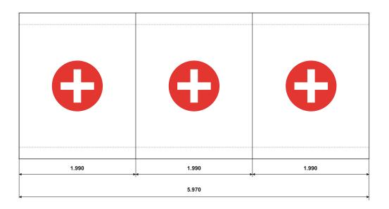
Three universal building segments form a pass-through tube for quick access and handling of the injured. The 27.5-tonne capacity design provides additional restraining mass.
