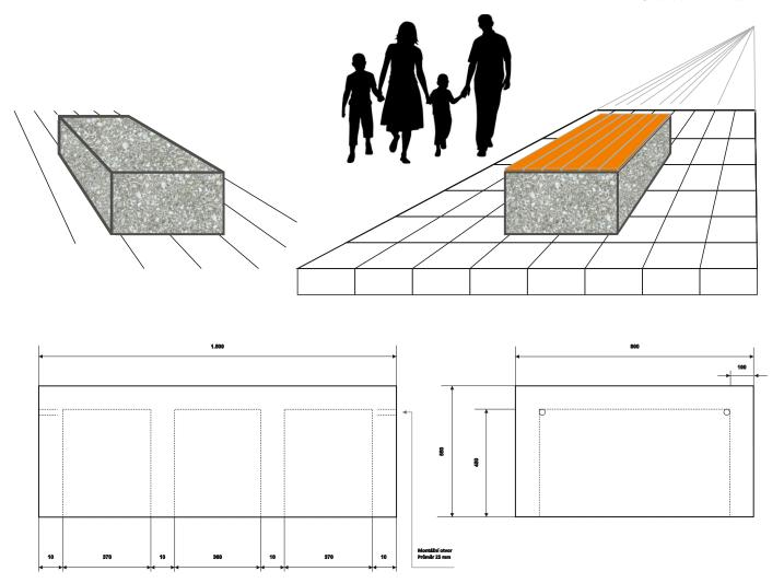
It is characterised by high resistance to the effects of blast pressure waves and to penetration by conventional projectiles, shrapnel and secondary shrapnel. Captures and diverts pressure wave. When anchored, it prevents a passenger vehicles from penetrating into the protected perimeter.
