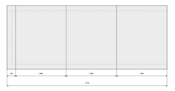
In the event of an explosion of the stored material, it directs the pressure wave out of the tubes, and reduce the risk of concrete fragments flying around. The 31.5 tonne capacity design provides additional restraining mass. The constructed sandbag containment berm will limit the velocity of projectiles, secondary shrapnel and pressure waves. Advantage of a quick assembly modular system.
