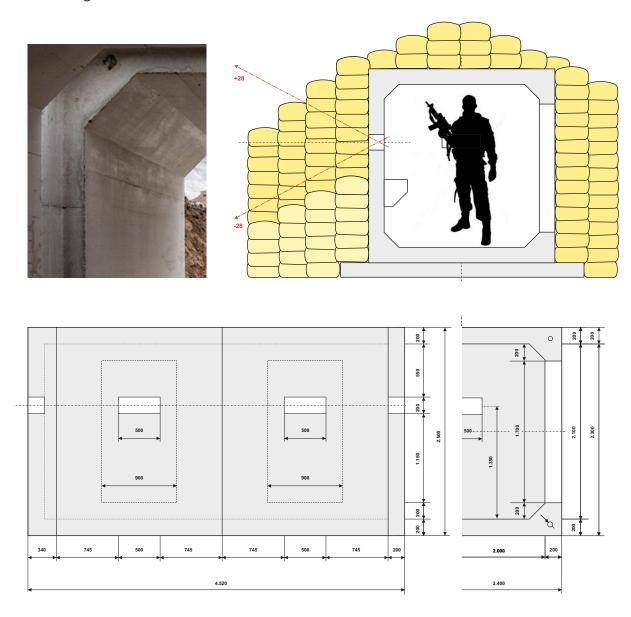
To increase the effectiveness of the protection, it is beneficial to partially embed it in the ground as part of the trench system and to reinforce the protection by lining it with natural material. Variably fitted universal building segment with embrasures, observations slits, entrance hole. Advantage of quick assembly and modular assembly to create a complex defence system.
