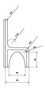
It is characterized by high resistance to the effects of the blast wave and to penetration by conventional projectiles, shrapnel and secondary shrapnel. Captures and diverts pressure wave, prevents the penetration of a passenger vehicle into the protected perimeter.
