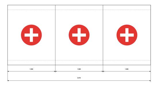
Three universal building segments form a pass-through tube for quick access and handling of the injured. The 27.5-tonne capacity design provides additional restraining mass.
