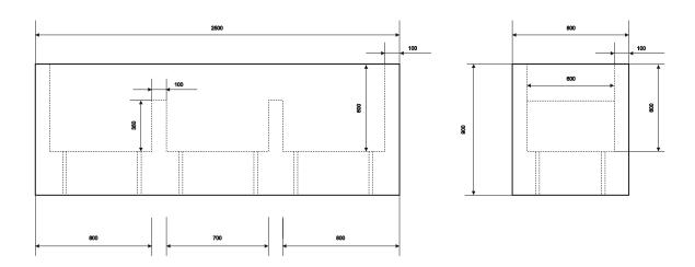
Either freestanding only the top part of the element, or placed on a plate based in the ground. The combination of the two parts, designed according to an explicit numerical simulation, has the ability to restrain the impact of a 20t truck driving at 100km/h.
