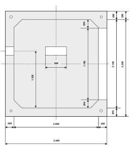
To increase the effectiveness of the protection, it is beneficial to partially embed it in the ground as part of the trench system and to reinforce the protection by lining it with natural material. Variably fitted universal building segment with embrasures, observations slits, entrance hole. Advantage of quick assembly and modular assembly to create a complex defence system.
