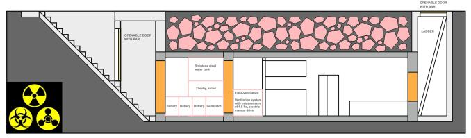
A sample of possible configuration. Five individually fitted segments with doors and escape exit.
